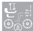
Quick stroke adjustment adjustable by dial activated by knee switch - with simultaneous speed limitation according to the foot stroke and feeding length
