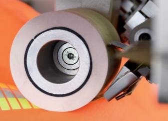
Hot-air welding machine for process reliable welding of reflective strips on work, sports, protective and saftey wear
