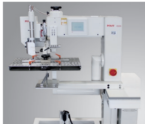
PFAFF 8320-020/061 Hot-air welding machine with adjustable tube guide
